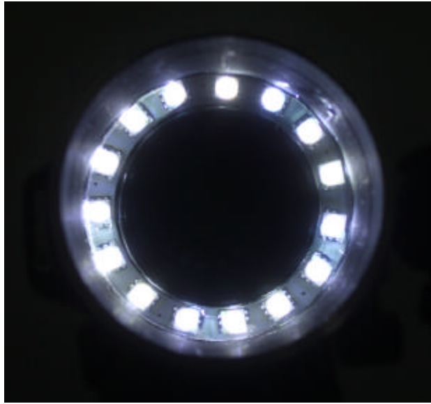
Fig 2. Internal Illuminator ring of the TiVi Camera Microscope adapter comprising 15 light emitting diodes emitting linearly polarized light.
