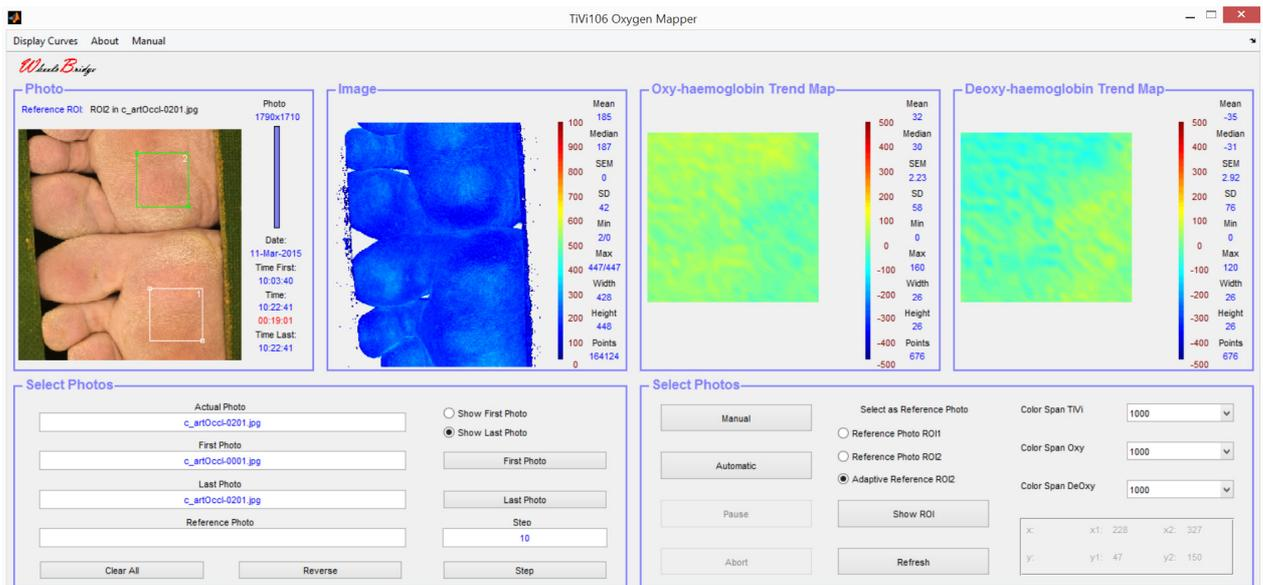
12. Note that the **Adaptive Reference ROI2** radio-button is automatically checked indicating that the system will now use the values within the white region of interest as measurement values and values within the green region of interest as reference values in each photo in the sequence.
