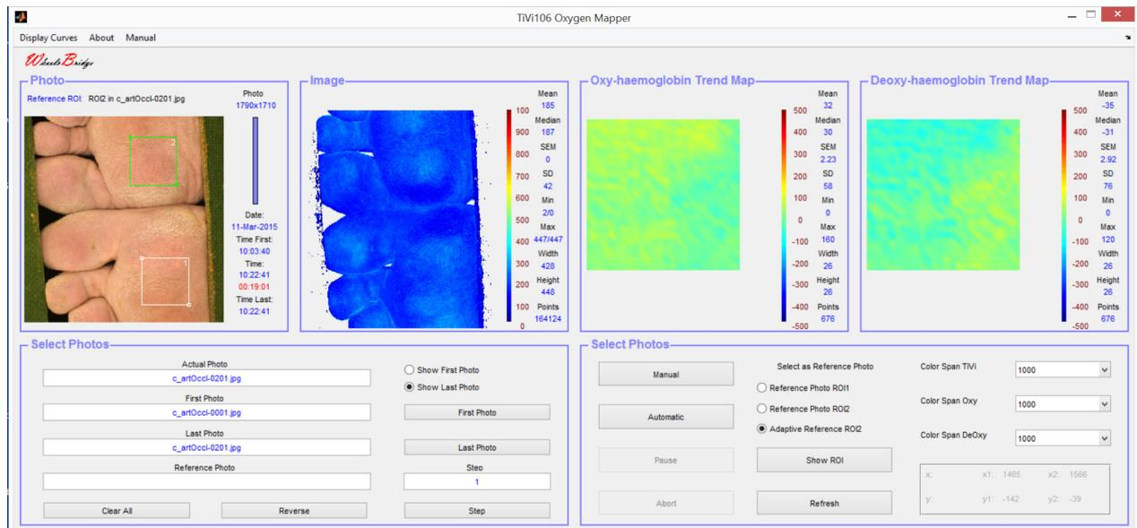
14. Select **Display Curves** in the pull-down menu to display the curves in a separate window. Note the movement artefacts in the measurement curve are balanced out by the same artefacts in the reference curve (the latter based on region of interest values in the reference foot not subjected to arterial occlusion).
