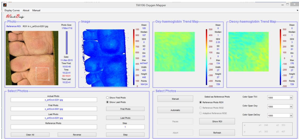
7. The reference area is now calculated as the average oxy- and deoxy haemoglobin concentration values within the actual region of interest and corresponding oxy- and deoxy-haemoglobin maps are displayed. To change the reference area to be calculated from the region of interest in the first photo click the **Show First Photo** radio-button and then click the Reference **Photo ROI1** button.
