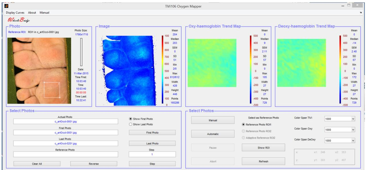
8. Click the **Automatic** button to scan through the photos in the sequence (and calculate the corresponding average oxy- and deoxy haemoglobin concentration changes).
