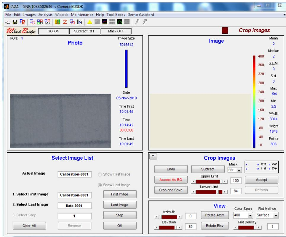
13. The width of the object displayed is now 10 mm which corresponds to a **Width** of 3044 pixels (displayed in lower right corner of the **Image** panel). The calibration factor for this particular *TiVi Microscope* setup is therefore 10.000 micrometers per 3044 pixels or 3.29 micrometers per pixel.
