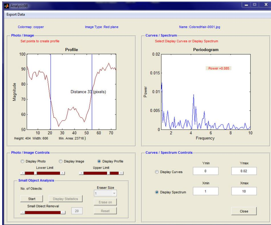
18. The diameter of the hair sample can now be read to be 33 pixels corresponding to 99 micrometers provided the TiVi microscope has been calibrated to 3 micrometers per pixel.
