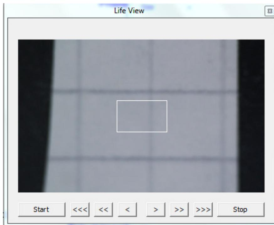
6. Adjust the focus with the **Arrow** buttons in the **Life View** window.
