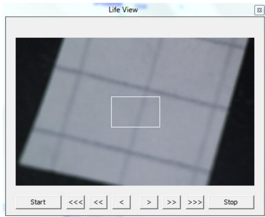
5. Rotate the object by turning the sample holder until the lines are parallel with the sides of the display window.
